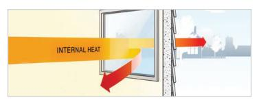
In particular during winter, Low E glass reflects heat back into the room, so less heat is lost through the windows. In summer, the sunis heat is reflected back outside.
