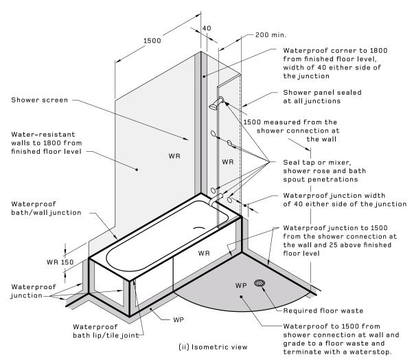
NOTE: All floor waterproofing to terminate at a waterstop.
