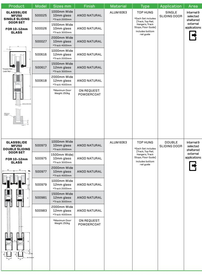
NOTE: System can be used in single, bi-parting and multiple lines of sliding doors. In ground channel guide systems available on request.
