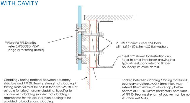
**NOTE:** For PF150 clamps connected to steel/concrete and bearing on timber cladding, facing material and/or timber packers, clamp spacing and balustrade height must be selected in accordance with timber substrate requirements in design tables.
