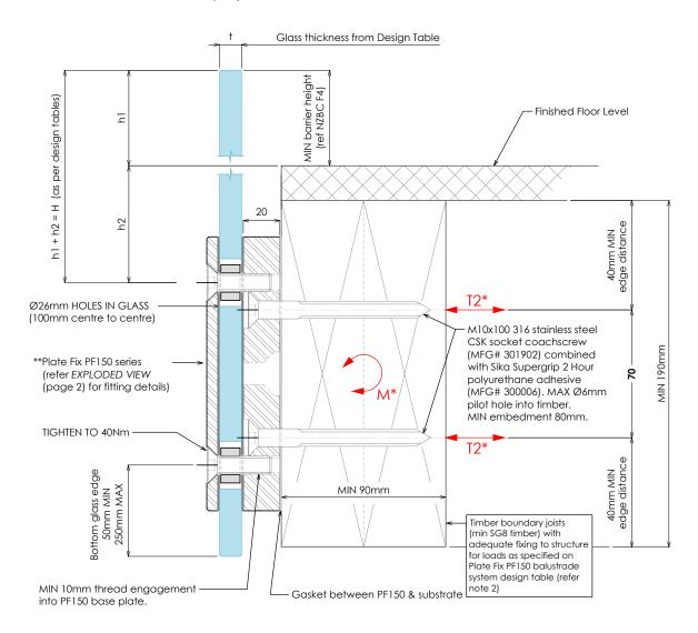
Refer to Plate Fix PF150 balustrade system design table for required glass thickness, fixing spacings and fixing loads according to AS/NZS 1170.1:2002 for the occupancies listed above. Refer to design tables and elevations for post failure requirements. Interlinking rail / clips not shown for clarity. 'H' refers to top of barrier.
