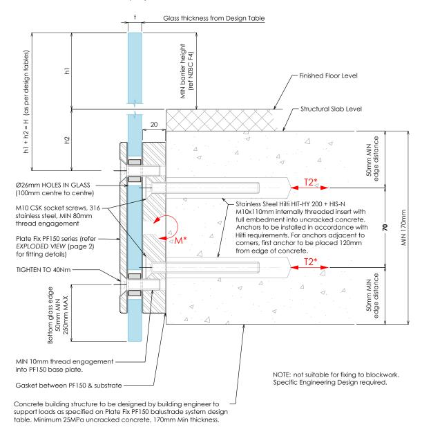
Refer to Plate Fix PF150 balustrade system design table for required glass thickness, fixing spacings and fixing loads according to AS/NZS 1170.1:2002 for the occupancies listed above. Refer to design tables and elevations for post failure requirements. Interlinking rail / clips not shown for clarity. 'H' refers to top of barrier.
