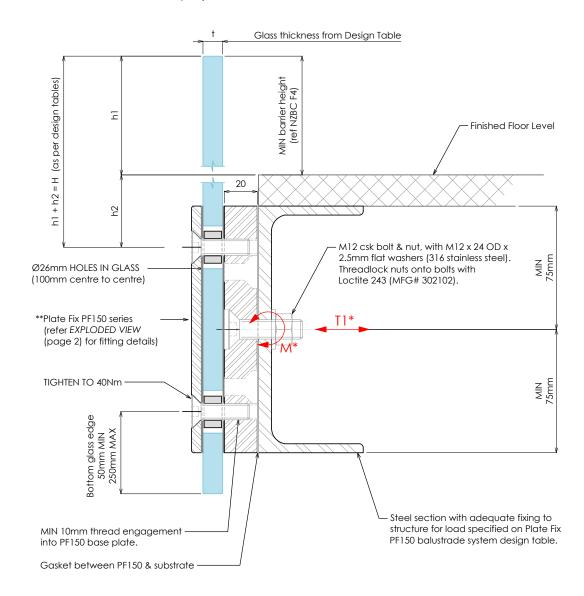
Refer to Plate Fix PF150 balustrade system design table for required glass thickness, fixing spacings and fixing loads according to AS/NZS 1170.1:2002 for the occupancies listed above. Refer to design tables and elevations for post failure requirements. Interlinking rail / clips not shown for clarity. 'H' refers to top of barrier.
