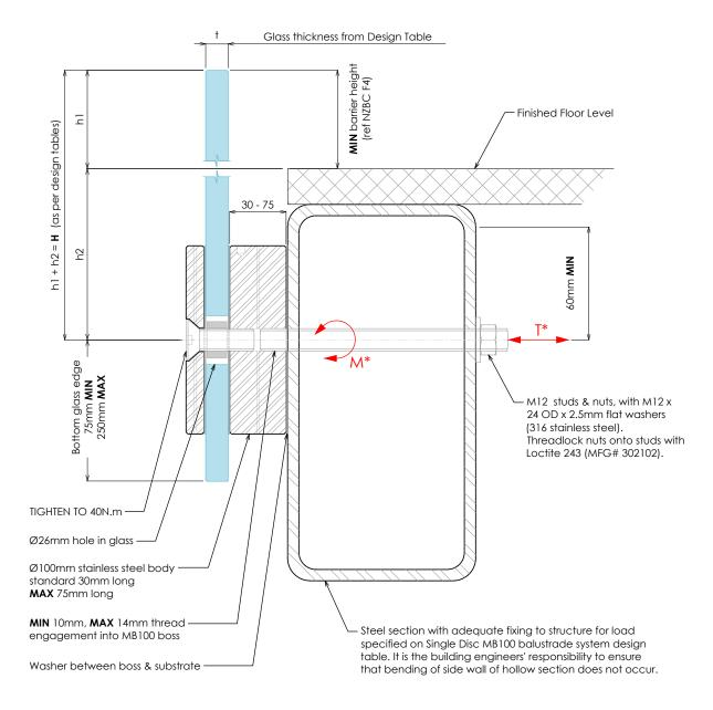
Refer to Single Disc MB100 balustrade system design table for required glass thickness, fixing spacings and fixing loads according to AS/NZS 1170.1:2002 for the occupancies listed above. Refer to design tables and elevations for post failure requirements. Interlinking rail / clips not shown for clarity. 'H' refers to top of barrier.
