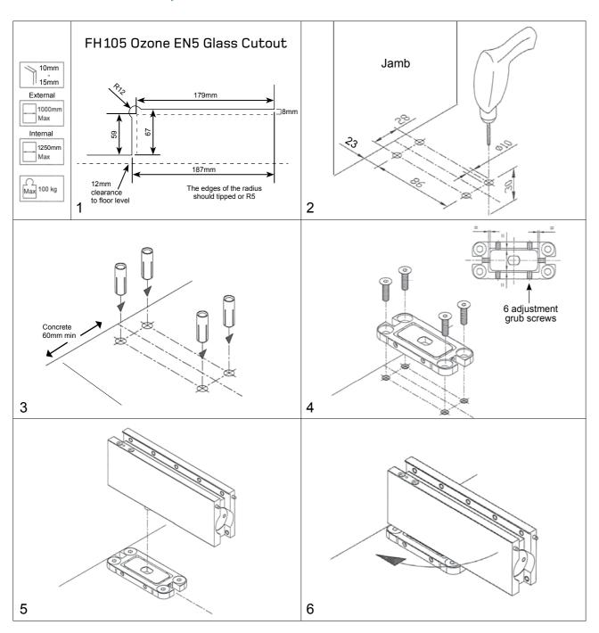
Once the patch is at 90° to the base the gaskets can be added and the door slid onto the patch and clamped in place by tightening
