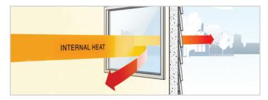
In particular during winter, Low E glass reflects heat back into the room, so less heat is lost through the windows. In summer, the sun's heat is reflected back outside.
