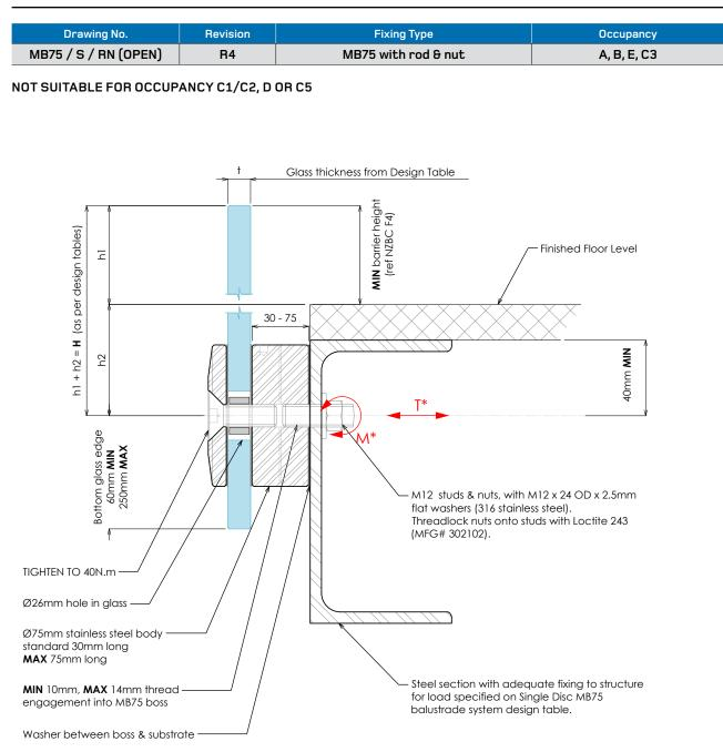
Refer to Single Disc MB75 balustrade system design table for required glass thickness, fixing spacings and fixing loads according to AS/NZS 1170.1:2002 for the occupancies listed above. Refer to design tables and elevations for post failure requirements. Interlinking rail / clips not shown for clarity. 'H' refers to top of barrier.
