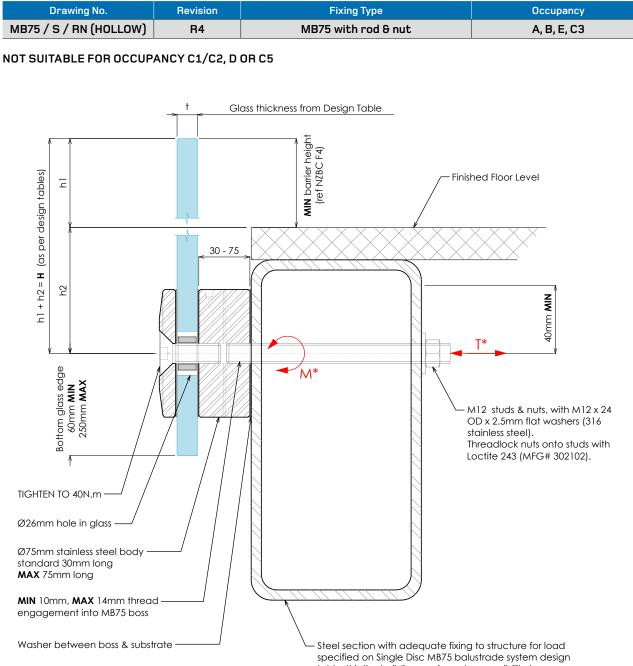
table. It is the building engineers' responsibility to ensure that bending of side wall of hollow section does not occur.
