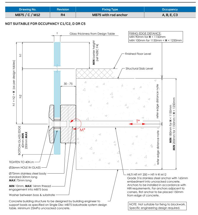
Refer to Single Disc MB75 balustrade system design table for required glass thickness, fixing spacings and fixing loads according to AS/NZS 1170.1:2002 for the occupancies listed above. Refer to design tables and elevations for post failure requirements. Interlinking rail / clips not shown for clarity. 'H' refers to top of barrier.
