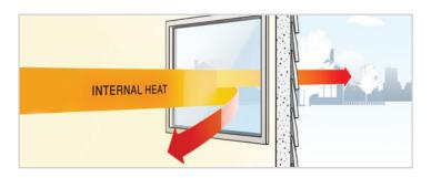
In particular during winter, Low E glass reflects heat back into the room, so less heat is lost through the windows. In summer, the sun's heat is reflected back outside.
