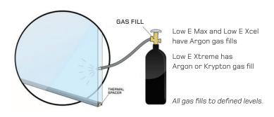
Low E double glazing performance is increased with the addition of a thermal spacer and gas.
