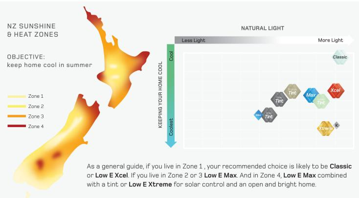
Notes: Keeping your home warm is measured by U Value Keeping Your Home Cool is measured by Solar Factor Natural Light is measured by Visible Light Transfer
