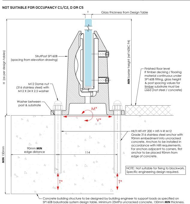
Refer to SP160B balustrade system design table for required glass thickness, fixing spacings and fixing loads according to AS/NZS 1170.1:2002 for the occupancies listed above. Refer to design tables and elevations for post failure requirements. Interlinking rail / clips not shown for clarity. 'H' refers to top of barrier.
