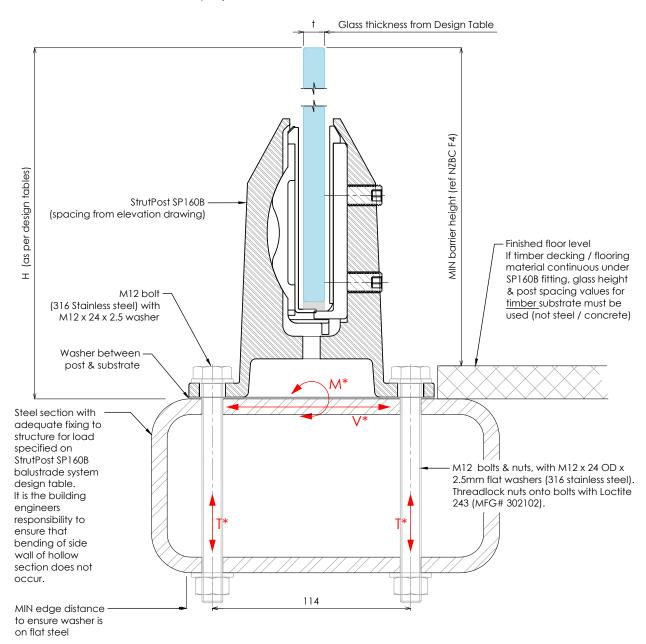
Refer to SP160B balustrade system design table for required glass thickness, fixing spacings and fixing loads according to AS/NZS 1170.1:2002 for the occupancies listed above. Refer to design tables and elevations for post failure requirements. Interlinking rail / clips not shown for clarity. 'H' refers to top of barrier.
