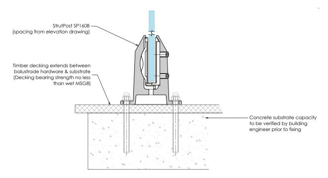
NOTE: TIMBER DESIGN TABLE VALUES MUST BE USED NOT STEEL OR CONCRETE
