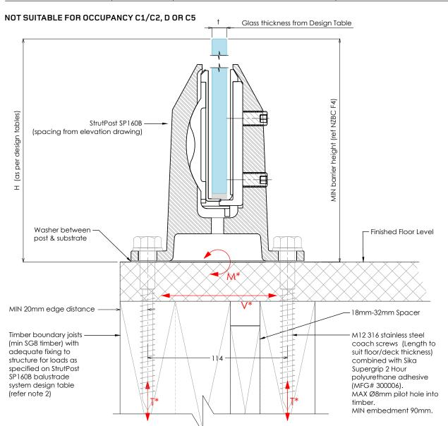
Refer to SP160B balustrade system design table for required glass thickness, fixing spacings and fixing loads according to AS/NZS 1170.1:2002 for the occupancies listed above. Refer to design tables and elevations for post failure requirements. Interlinking rail / clips not shown for clarity. 'H' refers to top of barrier.
